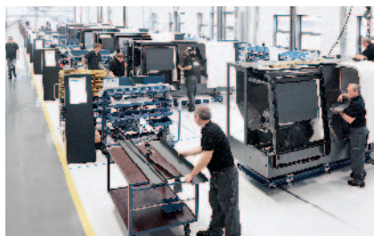
The new line assembly at GILDEMEISTER Drehmaschinen GmbH is put into operation. CTX and NEF machines can now be assembled in takt operation. Large assembly monitors at each takt station display the progress.
